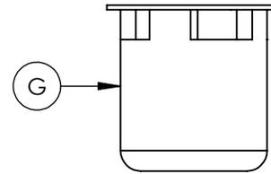
Insert the cup and trap (F&G). Push down firmly to ensure the trap is in the the bottom position.
