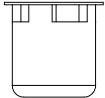
This waste provides a flow rate greater than 24L per minute under a 15mm water load. The flow rate can be seriously impaired if an adequate fall is not maintained throughout the length of the waste pipe.
