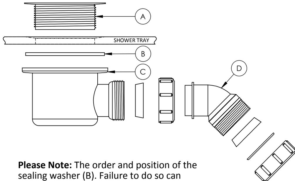
**Please Note:** The order and position of the sealing washer (B). Failure to do so can result in water leakage.
